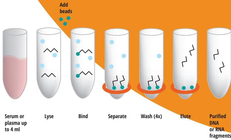
First, the uniquely formulated lysis buffer releases the circulating DNA from proteins and vesicles while DNases and RNases are inactivated. After binding of the DNA to the magnetic beads, they can be separated from the lysate with a magnetic plate. Following a few rapid wash steps to remove trace contaminants, the purified DNA is eluted from the magnetic beads using an Elution Buffer.
